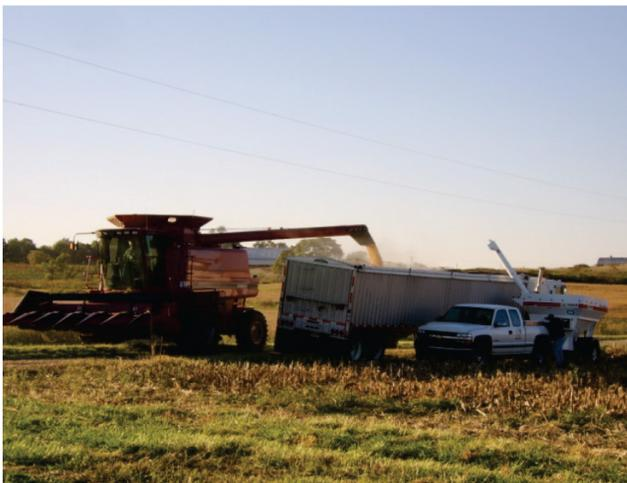
Figure 2. A grain cart equipped with scales or a weigh wagon is often used to quickly weigh loads for the mass flow sensor calibration procedure.
