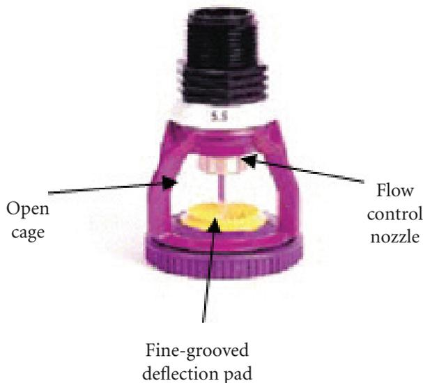
**Figure 7. Picture of low pressure spray nozzle with an open cage and fine-grooved deflection pad to prevent solids buildup on the pad, and a flow control nozzle to maintain appropriate pressure in rolling terrain.**
