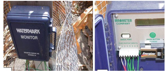
Figure 5A and B. Watermark Monitor datalogger. Up to eight Watermark sensors can be connected to the datalogger to monitor matric potential continuously.
