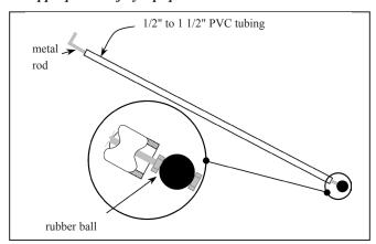
Figure 5. PVC pipe sampler.
