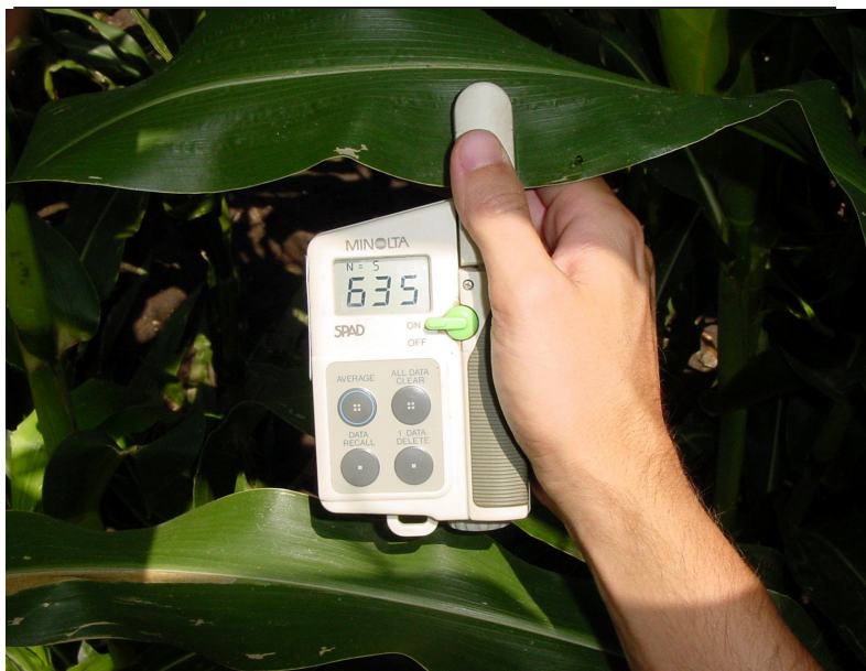
Figure 10. Hand-held chlorophyll meters are clamped over a leaf to measure light transmittance through a leaf.
