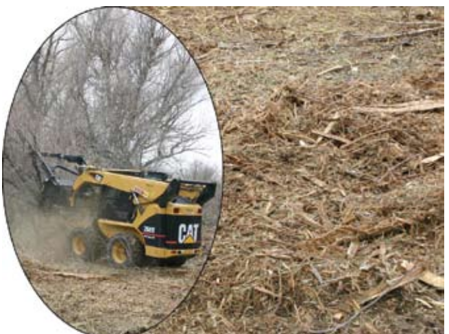
Figure 10. Russian olive tree being shredded with a chipper (left); chips covering the stump prevent stump treatment with an approved herbicide (right).
