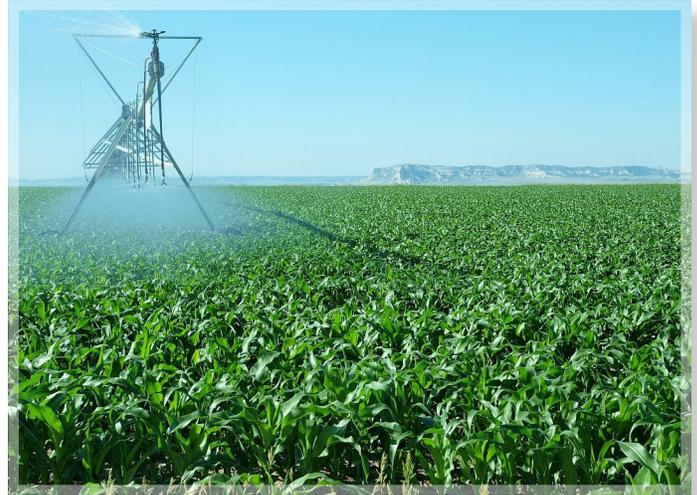
Center pivot irrigation systems, such as this one on a corn field, is a common method of delivering irrigation water. (Photo/Gary Stone)
