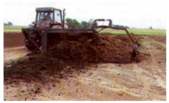
Figure 1. Turning of a composting windrow.
