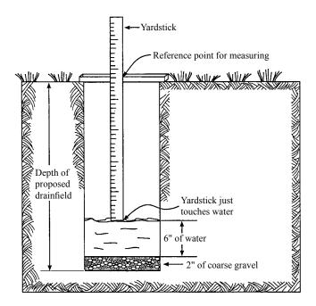
Figure 1. Percolation test hole.
