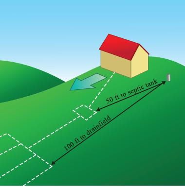
Figure 1. Locate wells at least 40 feet from any septic tank and at least 100 feet from any drainfield.
