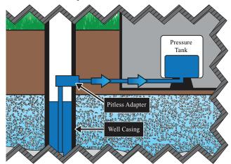
Figure 5. A pitless adapter attaches to the well casing and provides a watertight seal.
