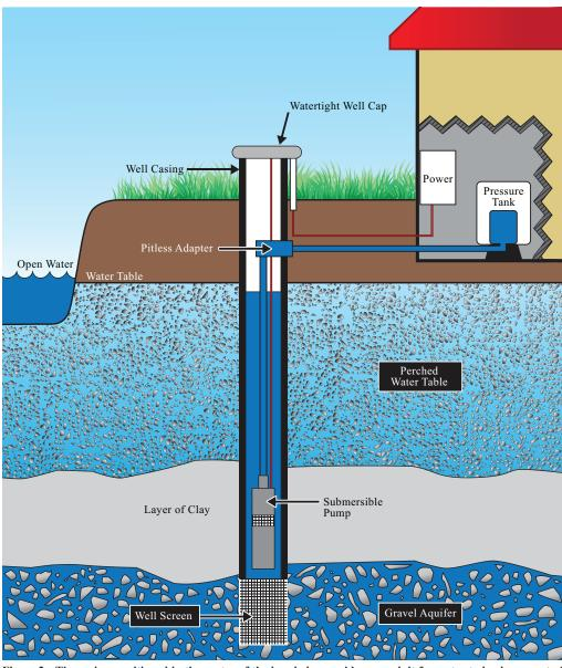
Figure 2. The casing, positioned in the center of the borehole, provides a conduit for water to be drawn out of the aquifer.
