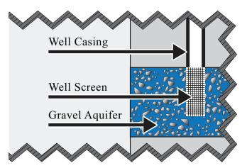
Figure 4. Water enters the well casing through a slotted well screen.
